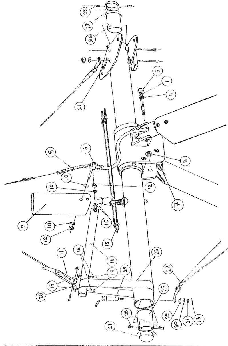
NOTE: ENSURE RESTRAINT STUD IS FULLY LOCATED THROUGH KEEL AND FASTENED WITH WING NUT BEFORE APPLYING WING TENSION
